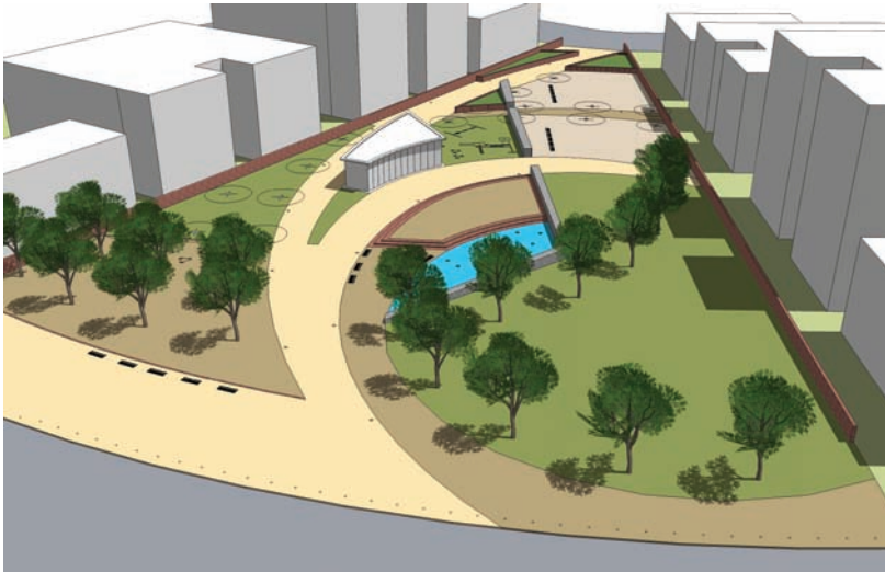
Fig. 19-9: The 2D edges are deleted and only the 3D trees remain, instantly populating the site plan with trees.
