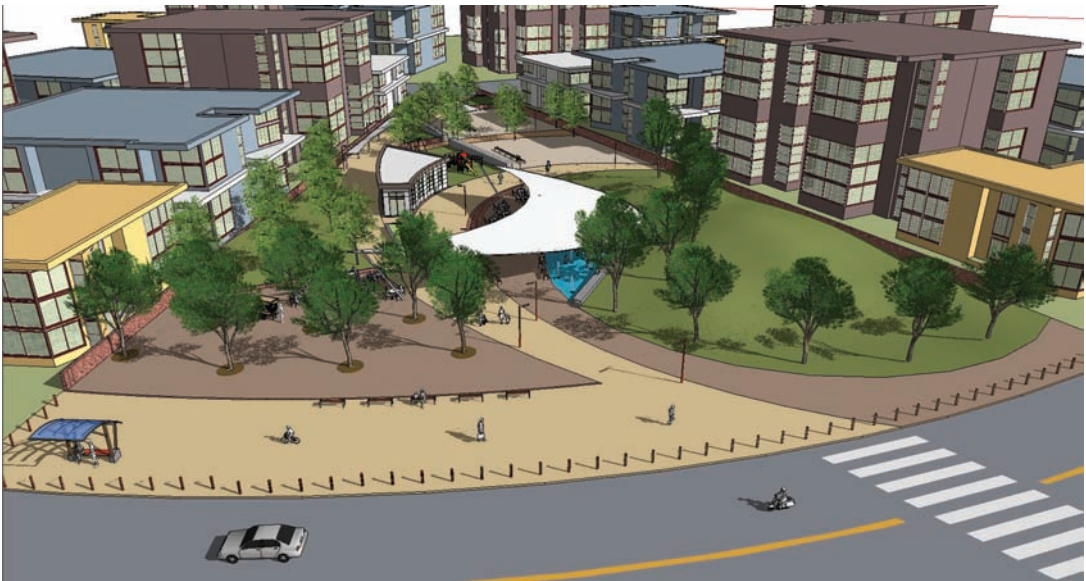
Fig. 19-60: Include cars and other vehicles to provide context, scale, and activity. Do not add too many vehicles because they can distract from a scene.
