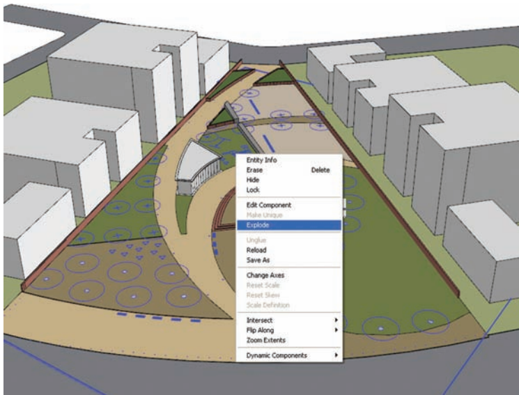
Fig. 19-4: Explode the imported Objects block/component.
