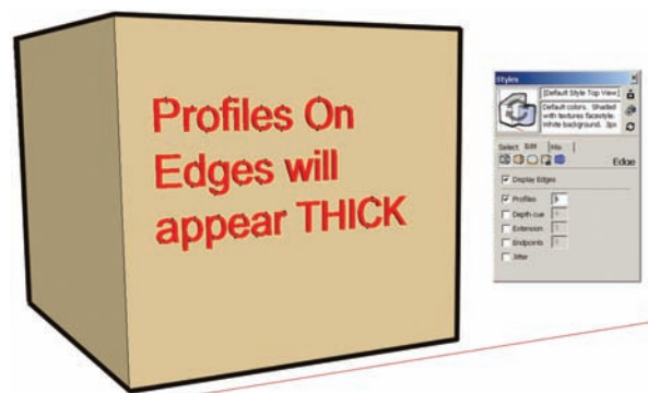
Fig. 2-21: Profiles are checked "on," displaying thicker edges.
