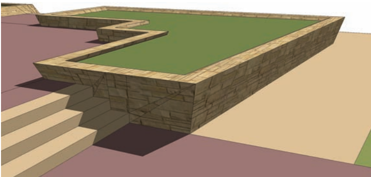
Fig. 7-50: The levered vertical faces of the wall.
