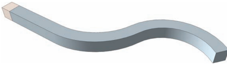
Fig. 8-10: Follow Me will Push/Pull the cube face following the path of the selected edges.
