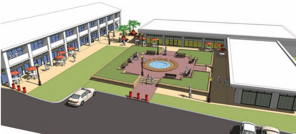
Fig. 10-14: Include pre-made components to complement the custom site furnishings. Include additional components such as tables and chairs, trash cans, cars, people, and water jets.
