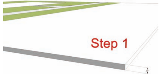
Fig. 6-16: Push/Pull the road surface downward 6".
