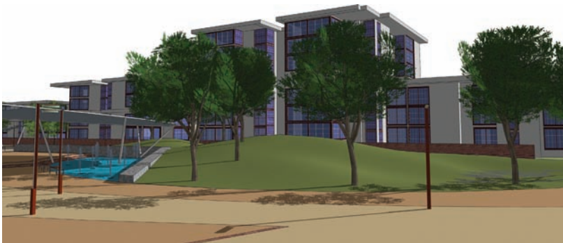
Fig. 19-37: The Smoove tool is then applied to the grid to generate slopes and contours. In this case, the slopes were snapped to the back of the wall adjacent to the water feature. Trees were dropped onto the slope using the Drop Ruby Scripts.
