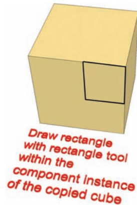
Fig. 3-5: In the component instance, draw a rectangle on the cube face as indicated.
