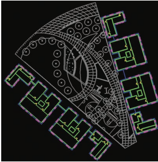
Fig. 17-6: The XREF Architectural file shows the building floor plans and footprint.
