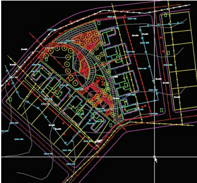
Fig. 16-1: An AutoCAD Base file filled with the relevant project information: architecture, civil, utility, survey info, and the site plan.
