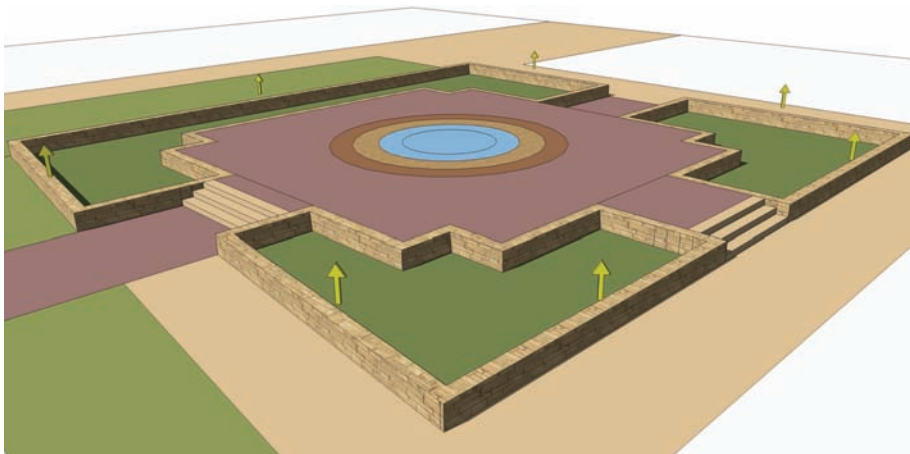
Fig. 7-35: Push/Pull the planter walls to match the plaza surface height.
